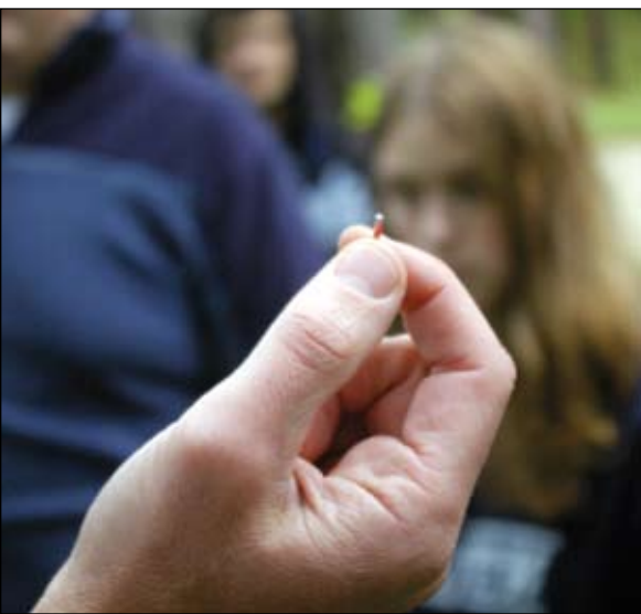
This tiny radio tag (ABOVE) is inserted just under the young sturgeons' skin. It emits a signal that can be picked up from quite a distance. This piece of equipment (BELOW) picks up the transmission from the tiny radio transmitters.
